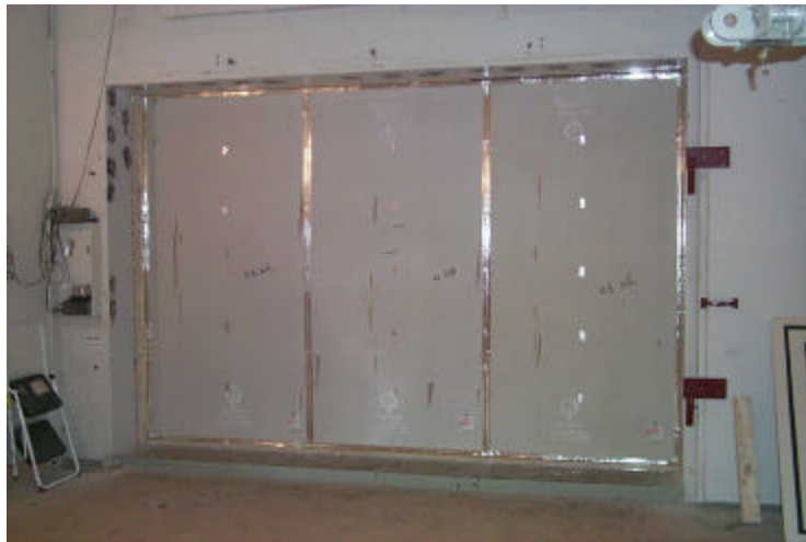
Figure 1: The Specimen B3414-5 installed in the IRC acoustical wall test frame.
