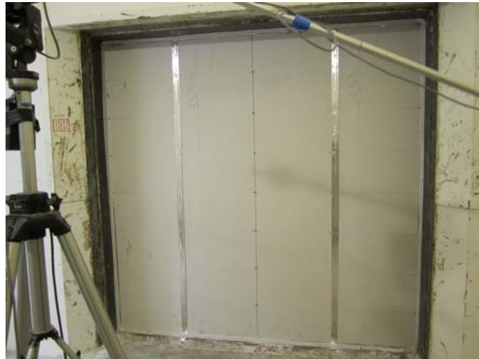
Figure 2: Photograph of source room side sheeting with staggered seams
